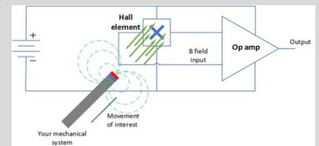
Hall sensors render precise and continuous measurements based on magnetic field strength. Within the Hall effect sensor, the Hall element sends the electric potential difference to an amplifier in order to make the change in voltage large enough to be perceived by the embedded system
